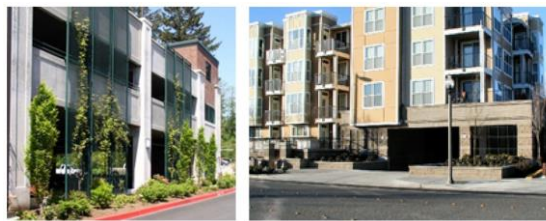
Figure 10.36.050(8)(b). The parking garage on the left includes decorative grillwork and vines to enhance its facade. The one on the right includes landscaping to separate the parking from pedestrians.
