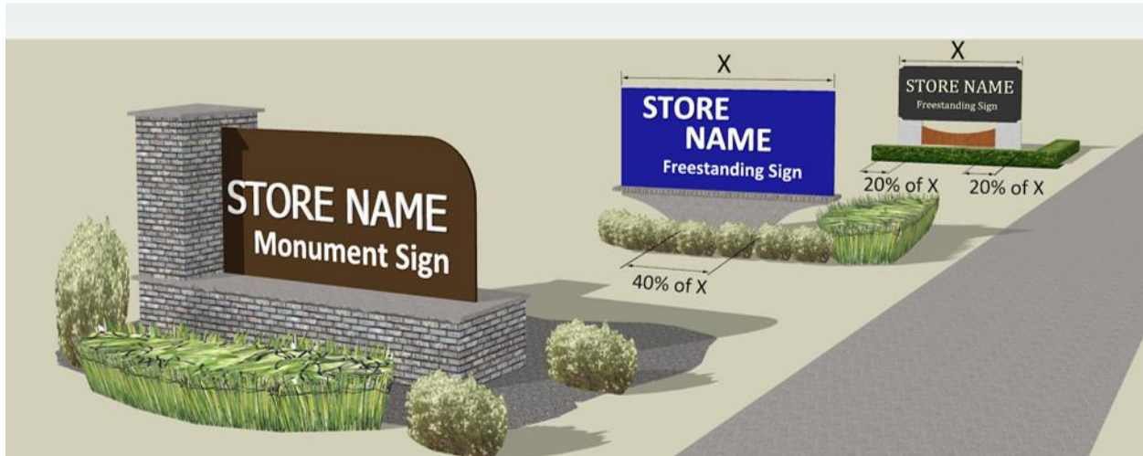
Figure 10.50.090(2)(a) Minimum ground anchoring provisions for monument signs.
